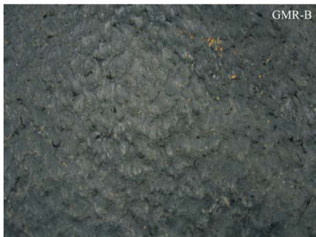
(b) Surfaces of rough geomembranes.
