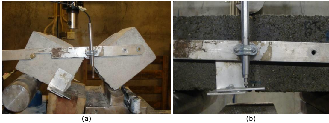
Figure 12 – Failure mode of the CEBs tested under three-point bending: (a) failure at the middle span of an air dry CEB; (b) crack tip initiation at the middle span of a CEB tested saturated.
