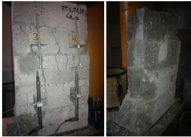
Figure 15 – Failure mode of a masonry prism constituted by CEBs manufactured with mixture SFA15.0.
