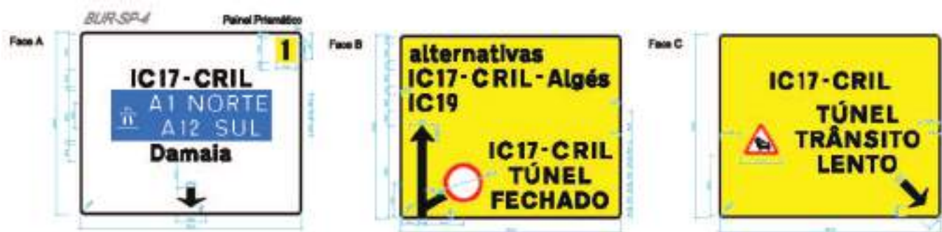
Fig. 15 Esquema ilustrativo das 3 faces dos painéis prismáticos. Illustrative scheme of the 3 faces of the prismatic reflectors.
