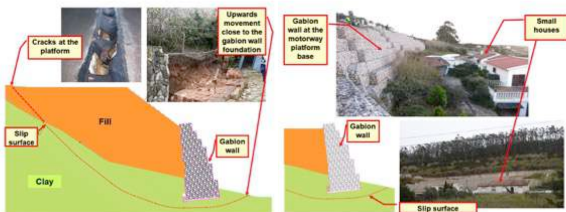
Figure 2. Slip surface below the gabion wall foundation.
