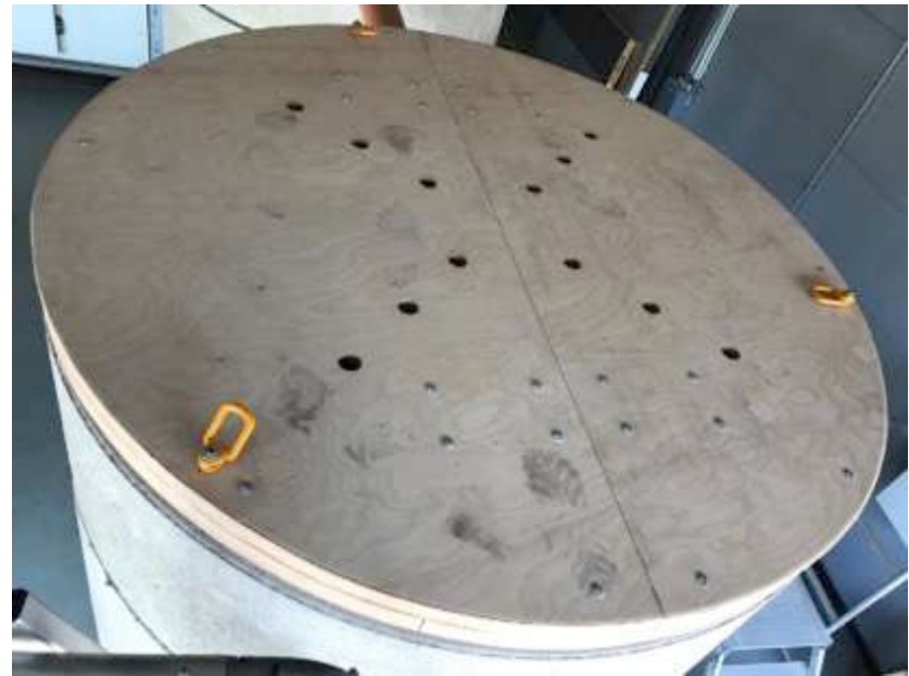
wooden plate with holes for dynamic probing tests
